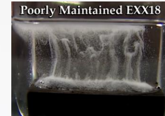
Low-Hydrogen Electrode (poorly stored)
